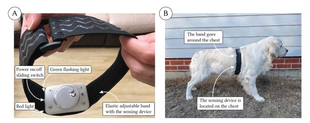
Fig. 1. *A:* The Patchkeeper device is attached to an elastic adjustable band. The device comes with two lights: a *green light* indicating whether the device is ON; and a *red light* indicating whether the device is in charging mode. *B:* The band can be strapped on the dog's chest.
